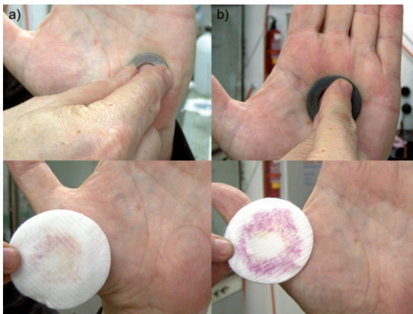
FIG. 3—Comparison of imprints intensities (developing reagent: triazine II) resulting from a 1-min contact with: (a) stainless steel ring, (b) uncoated iron ring.
